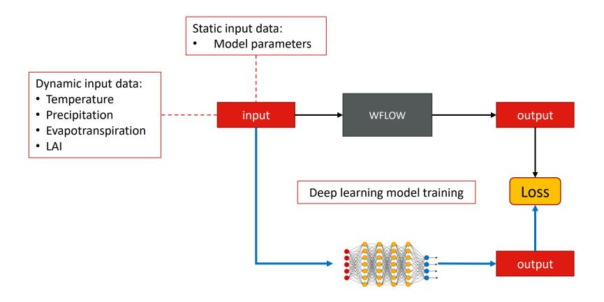
This step is needed to support a differentiable workflow and to save computational time
